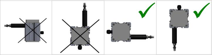
3. If there is a trickle of water (like a rain), the wire outlet must not be a drip of water upstream. If needed please use guide
